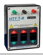
Designed to provide a fast, safe and reliable operational verification of Dielectric Withstand (hipot) and Ground Continuity Testers between calibration cycles. It allows the operator to check the result of the three failure modes encountered in production hipot and ground circuit testing (open ground, high leakage current, and dielectric breakdown) separately or in any combination to verify proper test equipment operation. HTT-1-B comes equipped with 3 5-way binding post banana compatible.
