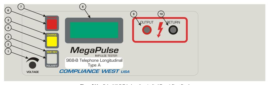
Figure 2 MegaPulse 968-B Telephone Longitudinal Type A Front Panel
