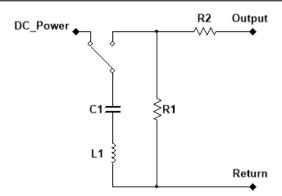
Figure 1 Telephone Longitudinal Type A Waveform Circuit Schematic
