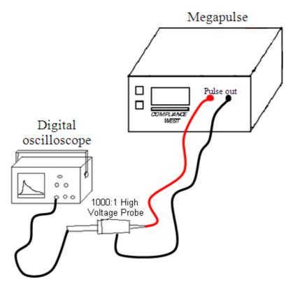
Figure 3. Waveform Measurement Setup
