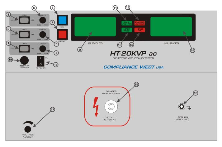
Figure 4-1. Front Panel Controls, Indicators and Connectors
