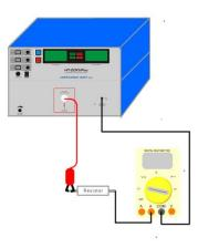
Figure 5-2. Current Measurement with 100 W High Voltage Resistor.
