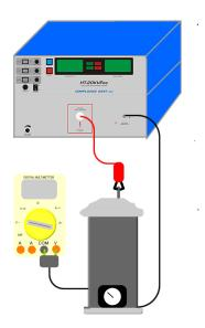
Figure 5-1. Voltage Measurement with 1000:1 High Voltage Probe
