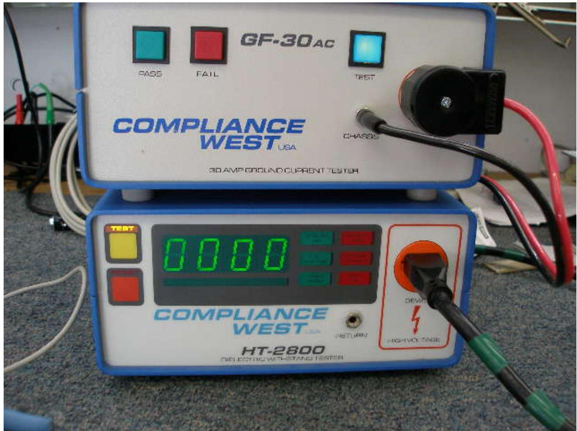
4. Take the other ends of the two wires and connect them to the rear panel of the HT Hipot tester as shown in the following picture. Note RED to RED, BLACK to BLACK. Also, connect the DB-9 on the rear panels of each tester together with the supplied cable.
