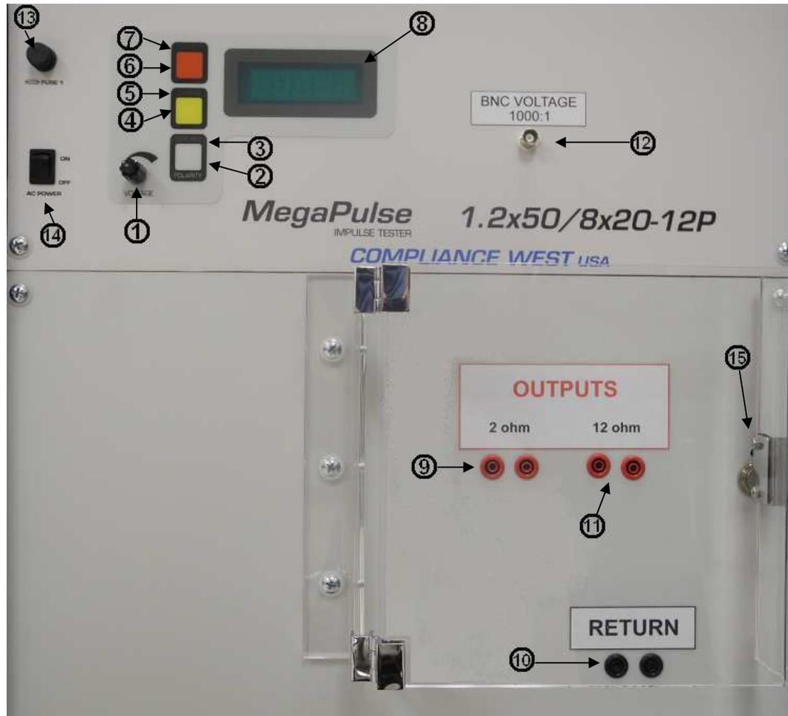
Figure 1. Controls, Indicators, Connectors – MegaPulse 1.2x50/8x20-12P 2/12 ohm Front Panel
