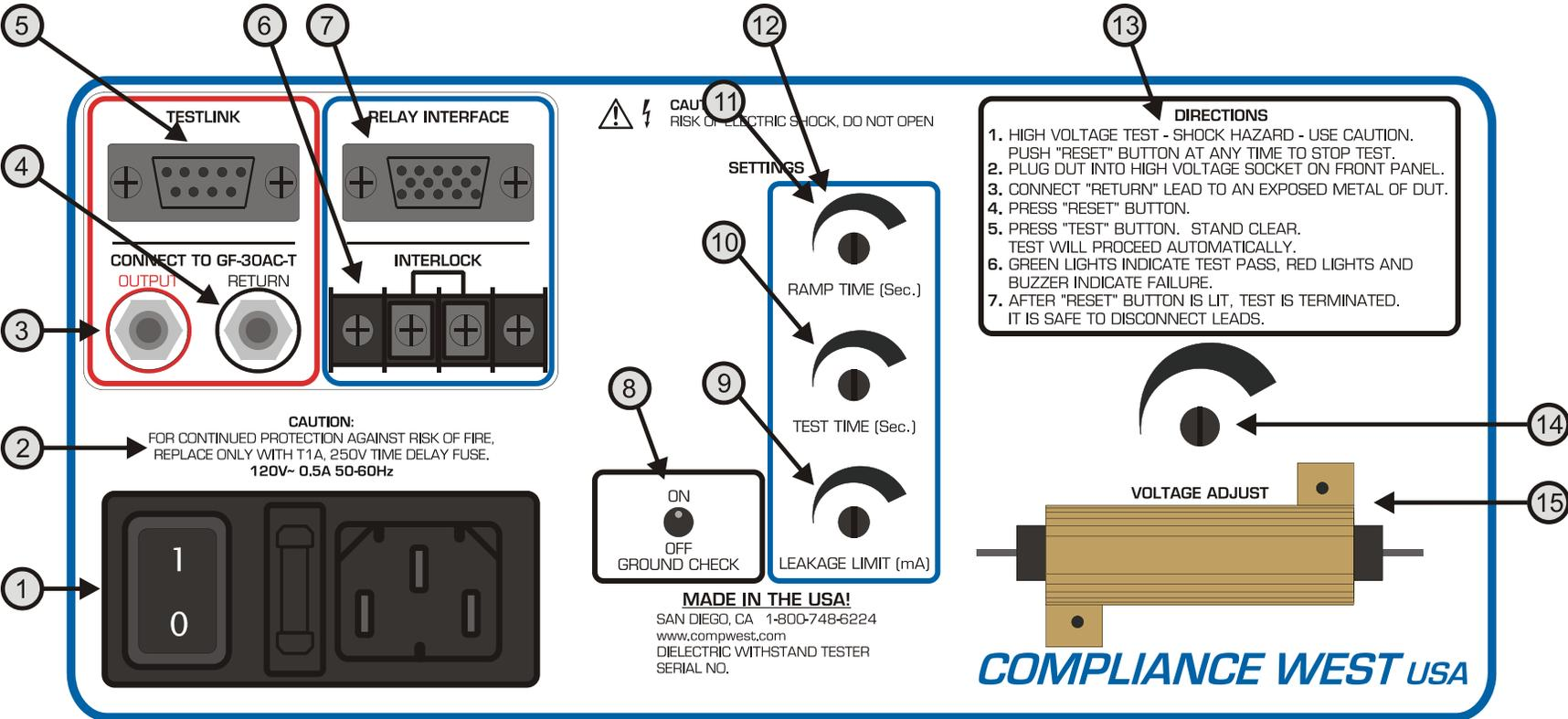
Figure 2. Rear Panel Controls, Indicators and Connectors
