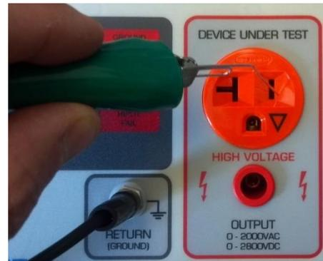
5. The test should immediately terminate with a buzzer. The **Ground OK, Ground Open, Full Voltage, Hipot Fail** and red **RESET** LED's should be lit.
