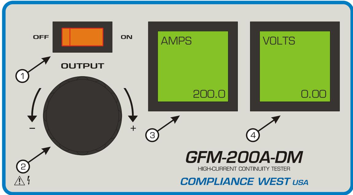
Figure 2-1. Controls, Indicators, Connectors - Model GFM-200A-DM Front Panel
