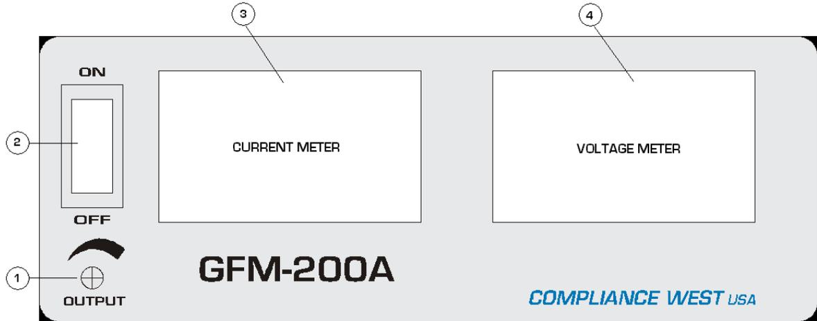
Figure 2-1. Controls, Indicators, Connectors - Model GFM-200A Front Panel
