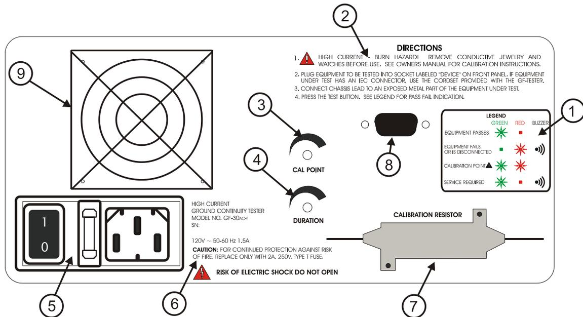
Figure 2-2. Control, Indicators, Connectors - Model GF-30AC-T Rear Panel
