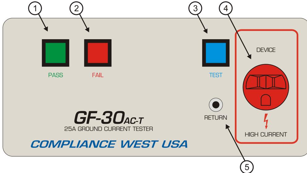
Figure 2-1. Controls, Indicators, Connectors - Model GF-30AC-T Front Panel
