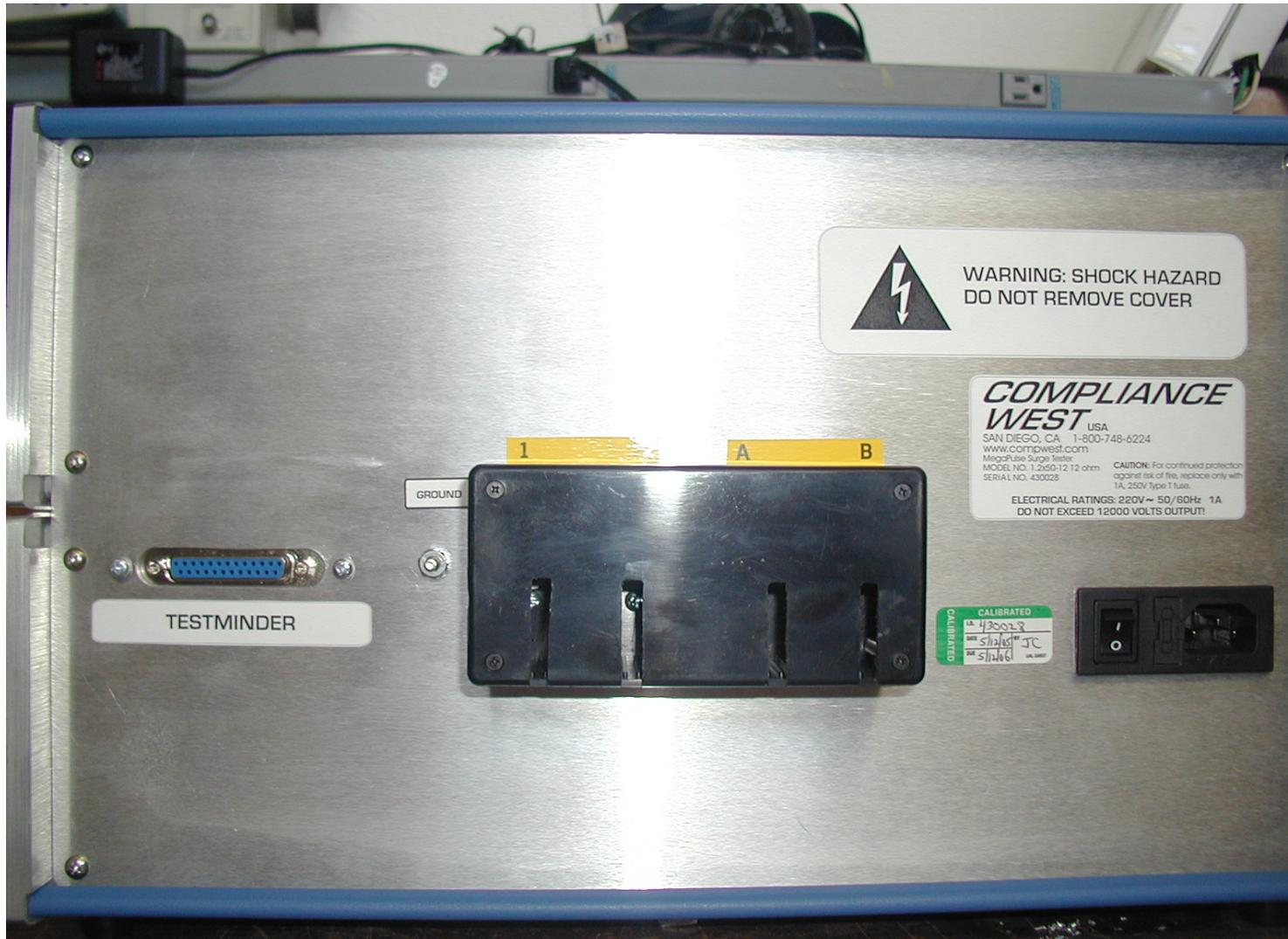
Figure 3 MegaPulse Option Connector Cover
