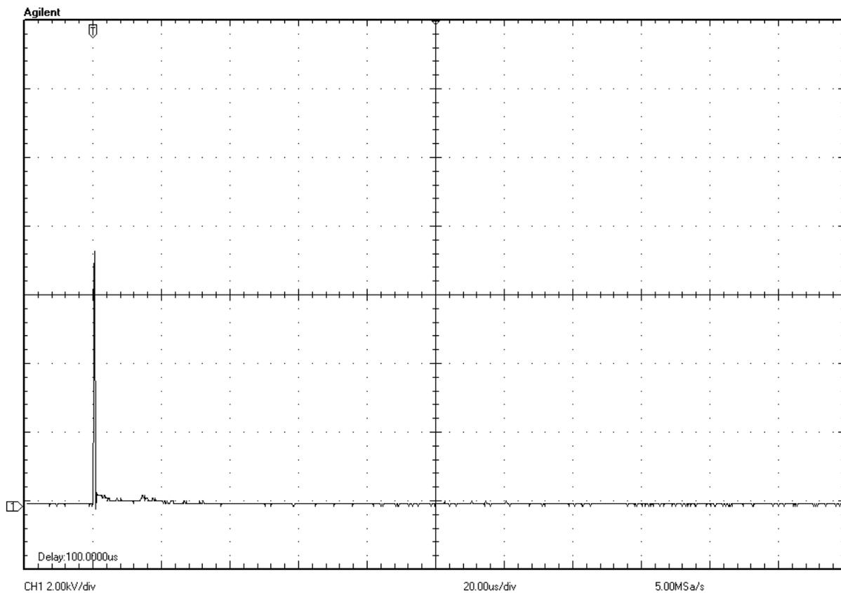
Figure 5: breakdown as the voltage is rising
