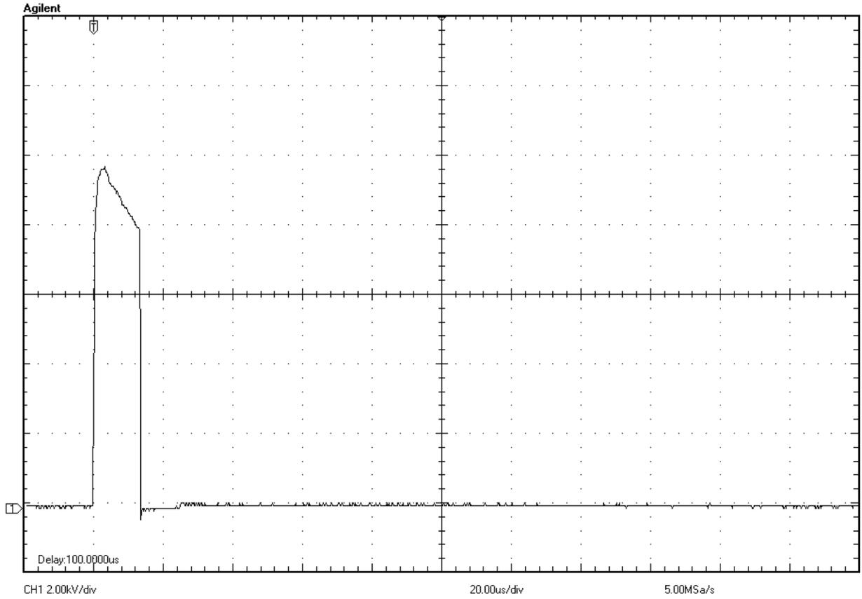
Figure 7: dielectric breakdown after V<sub>peak</sub> (delayed breakdown)
