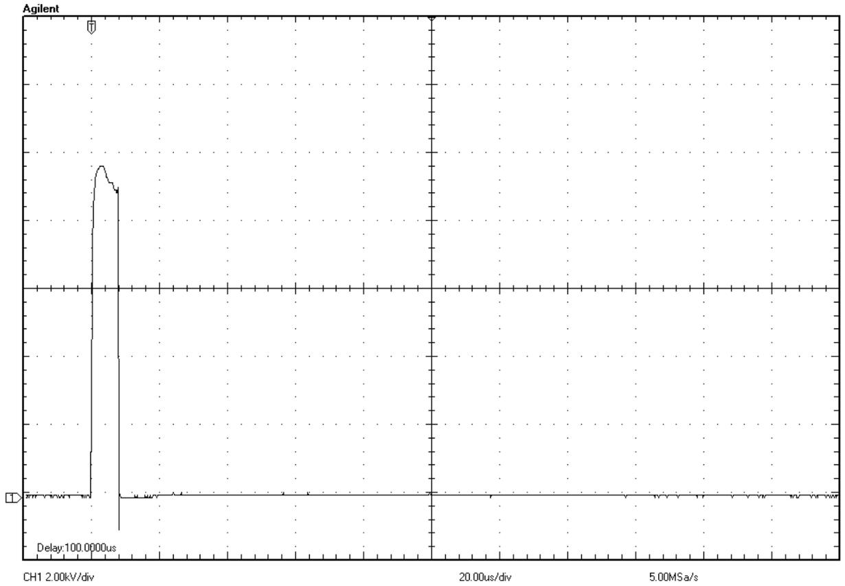
Figure 6: dielectric breakdown immediately after Vpeak
