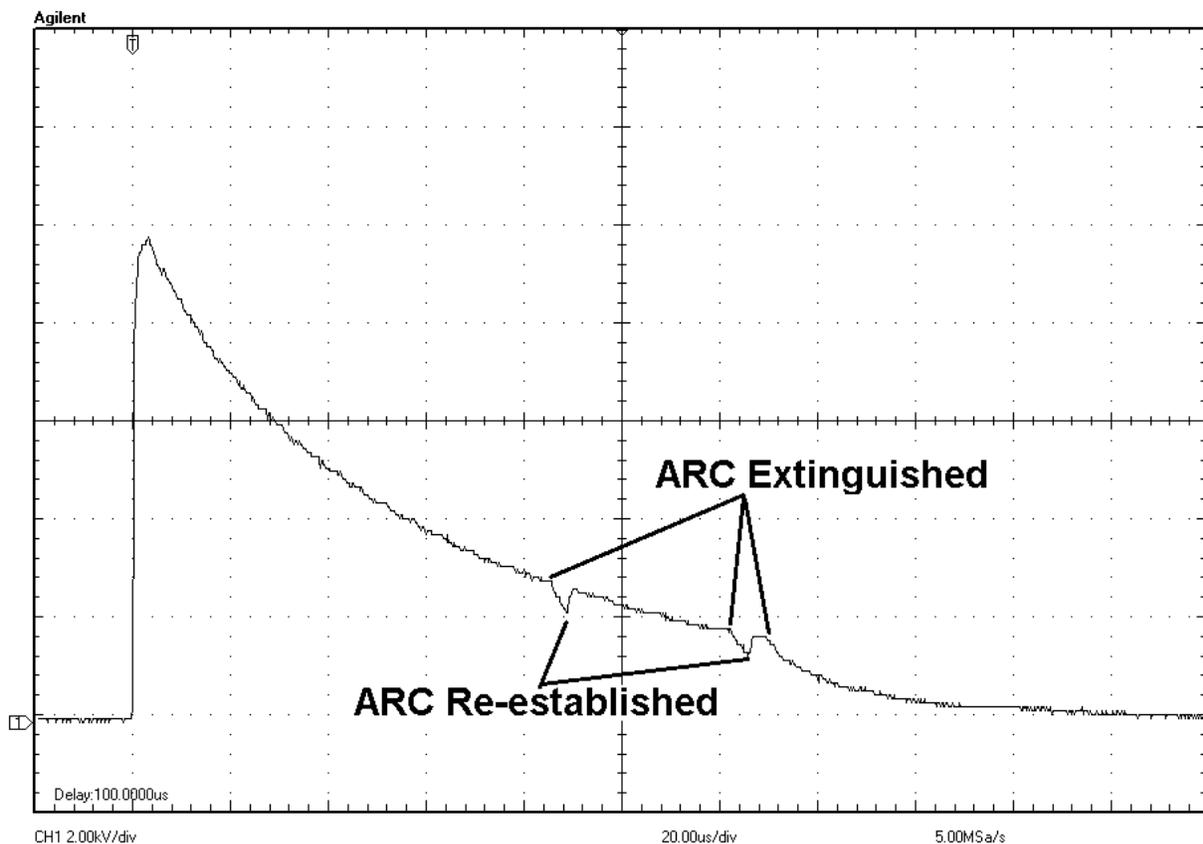
Figure 4: arc - extinguish - re-arcing cycle
