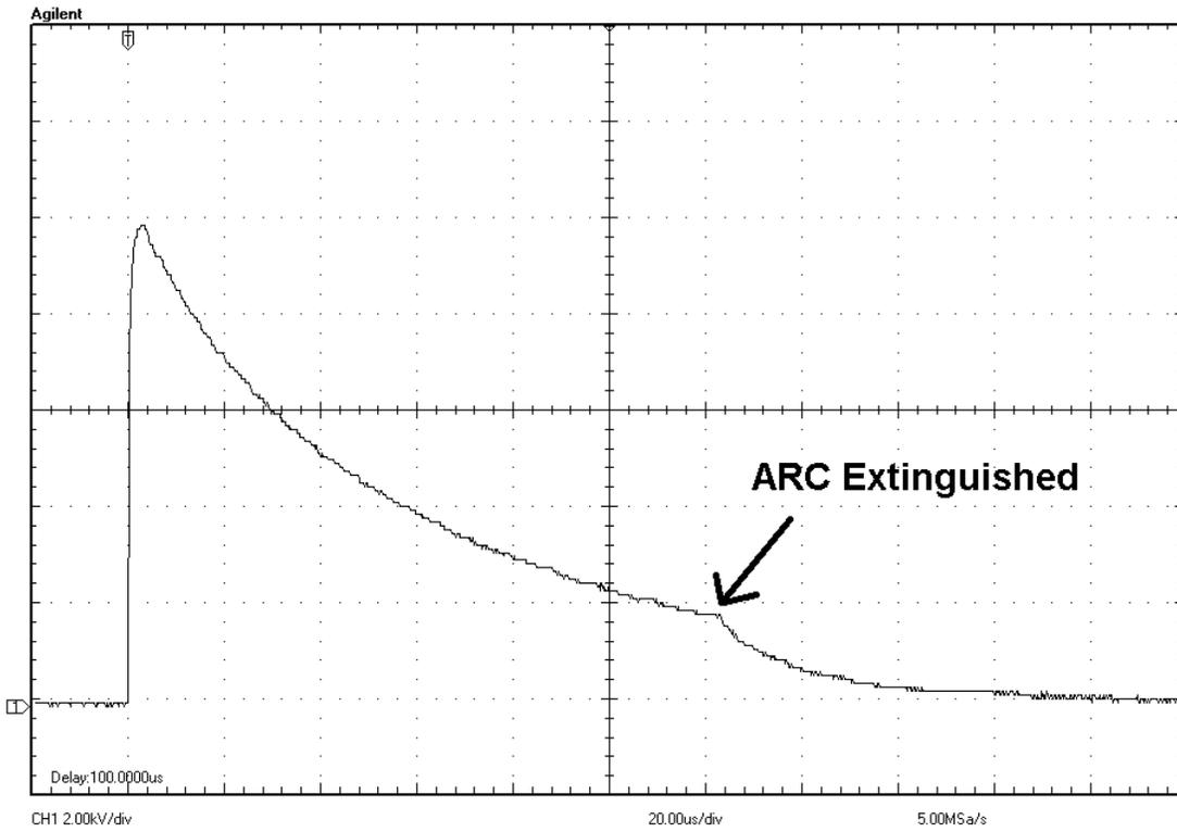
Figure 3: Actual output showing the arc being extinguished as the contact is closing
