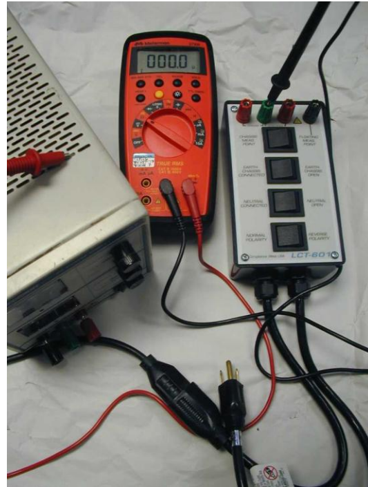
Figure 1 Grounding Circuit Continuity Test
