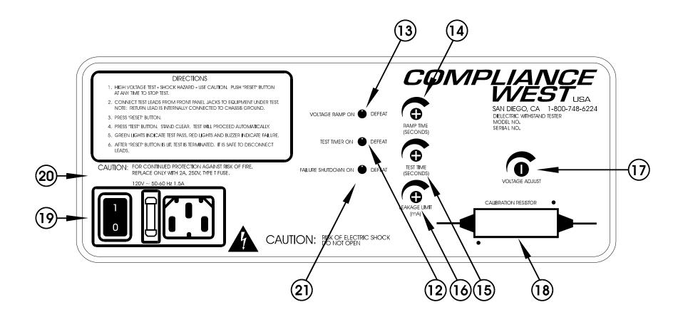
Figure 3-2. Controls, Indicators, Connectors - Model HT-5000ACAC 20mA Rear Panel
