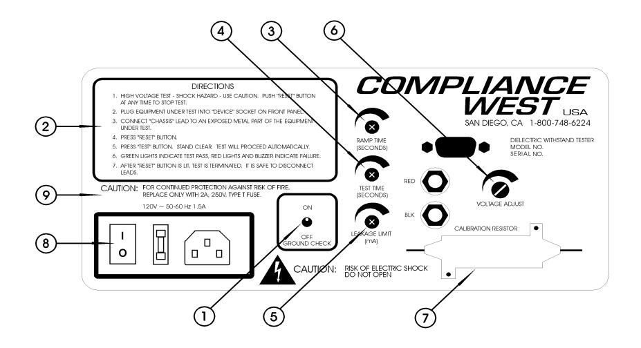
Figure 3-2. Controls, Indicators, Connectors - Model HT-3000 Rear Panel
