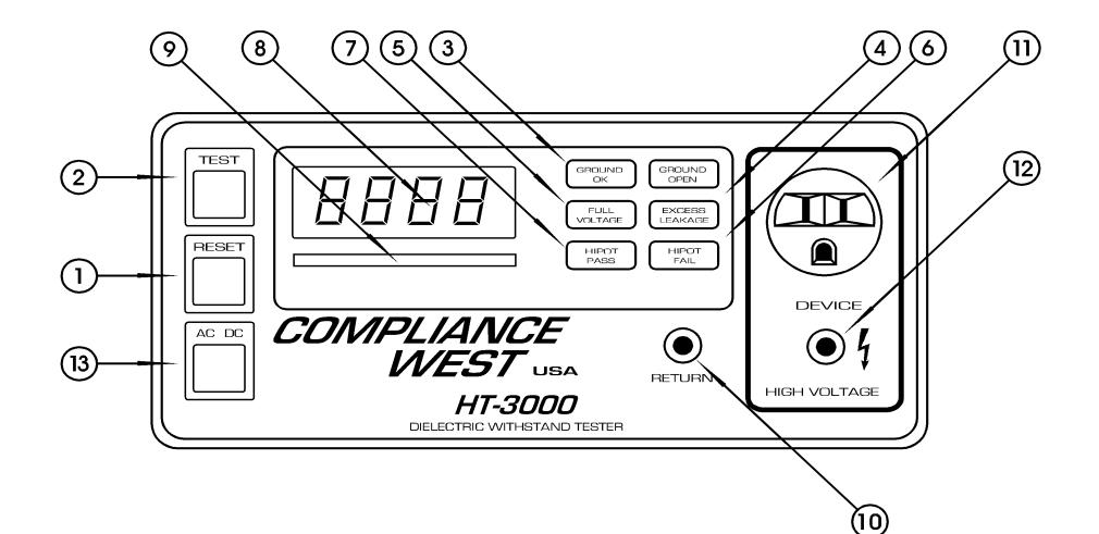
Figure 2. Controls, Indicators, Connectors - Model HT-3000 Front Panel
