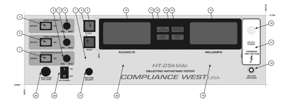
Figure 3-1. Controls, Indicators, Connectors - Model HT-25kVdc Front Panel
