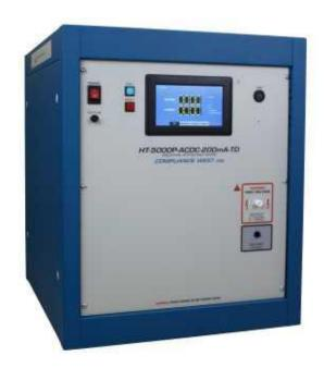
The tester has four test sequences that can be called from the screen or via USB control. A 7-inch color touchscreen monitors test progress and provides the user with output voltage, leakage current and elapsed test time during the test. Test results of Test Pass/Fail, maximum voltage and current delivered and test duration are displayed on the touchscreen after the test and can be sent via USB to network storage locations.
