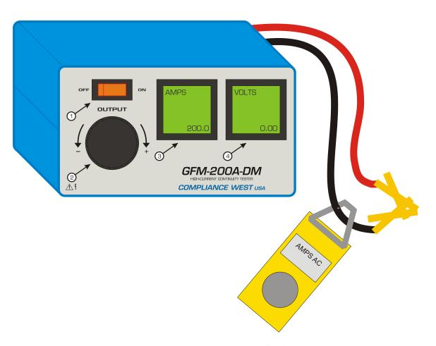
Figure 2-4. Current Test Verification set up
