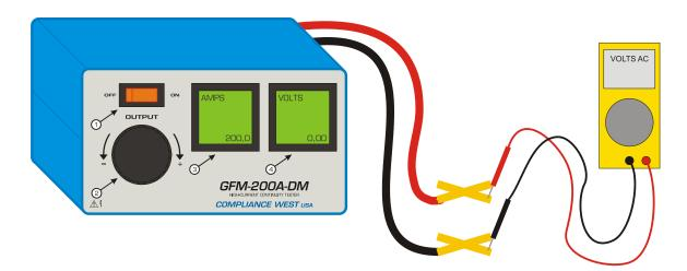
Figure 2-3. Voltage Test Verification set up
