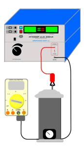
Figure 4-1. Voltage Measurement with 1000:1 High Voltage Probe
