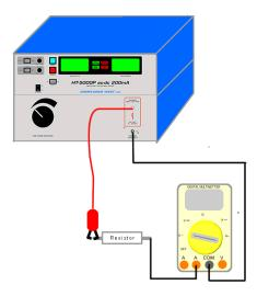
Figure 4-2. Current Measurement with 1000W High Voltage Resistor.
