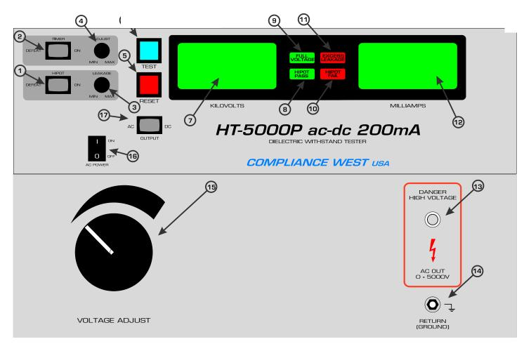
Figure 3-1. Front Panel Controls, Indicators and Connectors
