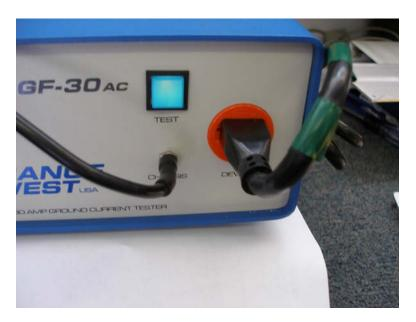
2. Take the other ends of the two wires and connect them to the 0.1 ohm resistor on the rear panel as shown below. We provide a connector for use between the ground of the cordset (middle connection) and the resistor with an alligator clip. In the nest step you will use a screwdriver as shown to set the red and green lights on the front panel to light simultaneously.
