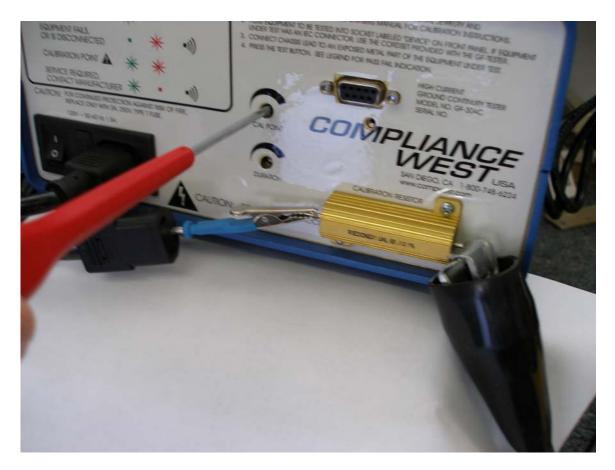
3. As shown below, push the test button and hold it while turning the screwdriver from side to side to get both the red and green lights to come on at once. This will set the GF-30ac to indicate test results properly.
