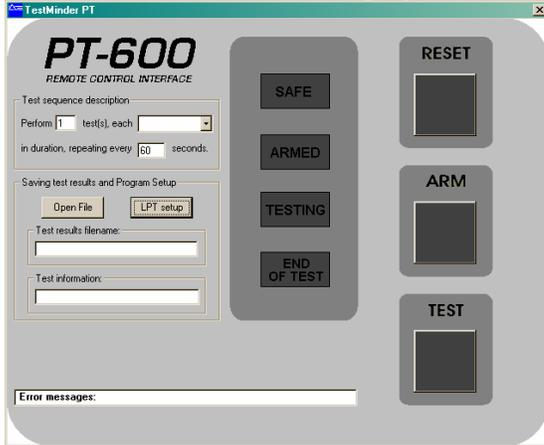
2. On the front of the PT-600, turn the Timer Knob at the top of the tester to the "AUTO" setting. If the knob is not set to the AUTO position, or if the Interlock circuit is not in the safe mode by all doors being closed, the TestMinder PT screen on the computer will gray out all the buttons. When the interlock is properly safe, and the Timer Knob is set to the AUTO position, the pictures of the buttons and lights will be shown in color.
