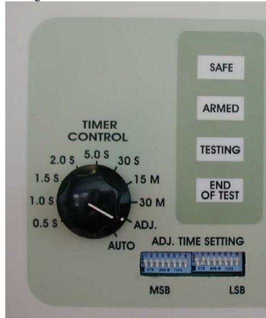
2. On the computer screen, set the number of tests and test period as above, but set the test duration to "Adj. Time Set".
