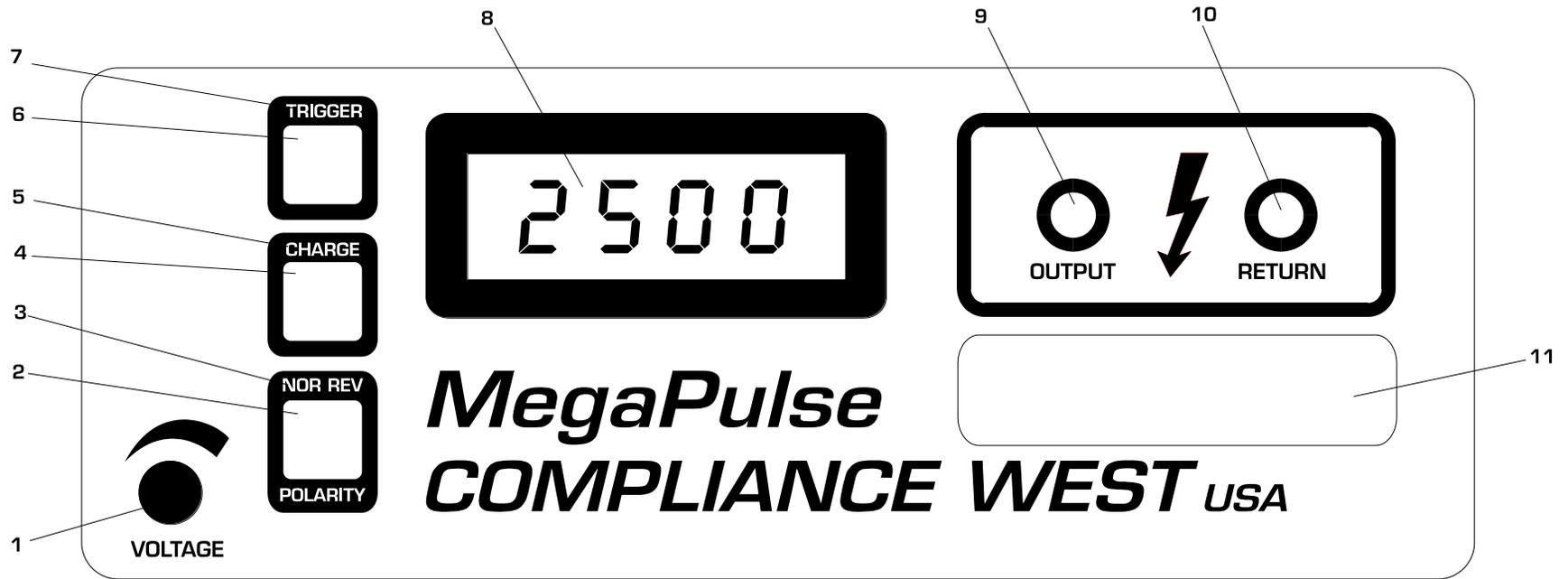
Figure 2. Controls, Indicators, Connectors – MegaPulse series Front Panel
