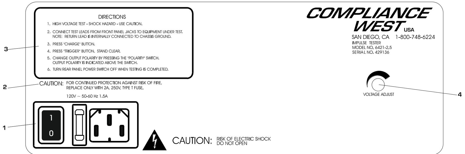
**Figure 3. Controls, Indicators, Connectors – MegaPulse series Rear Panel**
