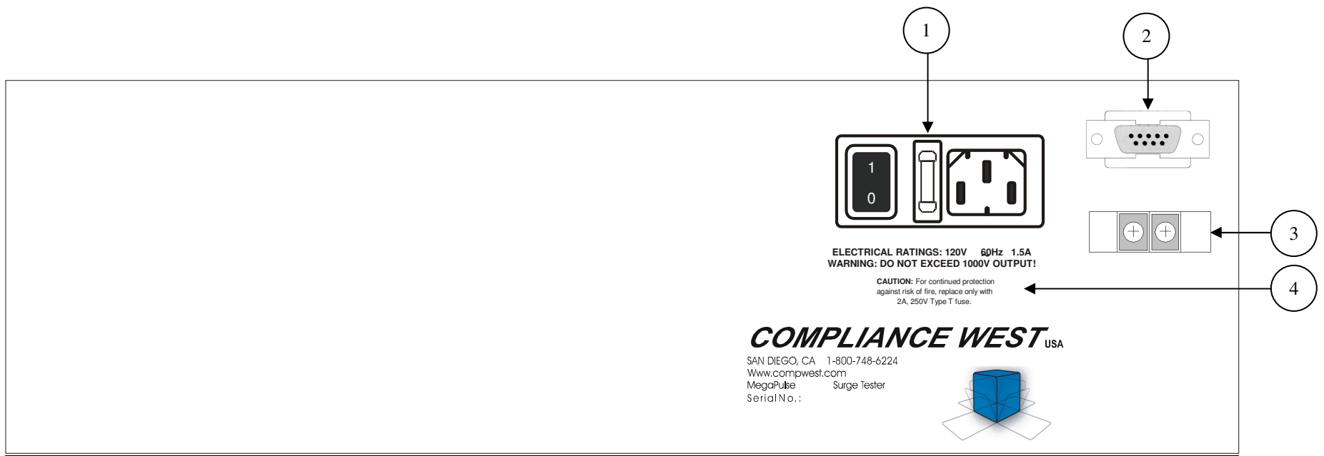
Figure 2. Controls, Indicators, Connectors – MegaPulse Defib Low Energy Rear Panel
