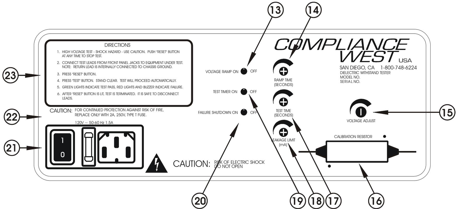
Figure 3. Controls, Indicators, Connectors - Model HT-5000P Rear Panel
