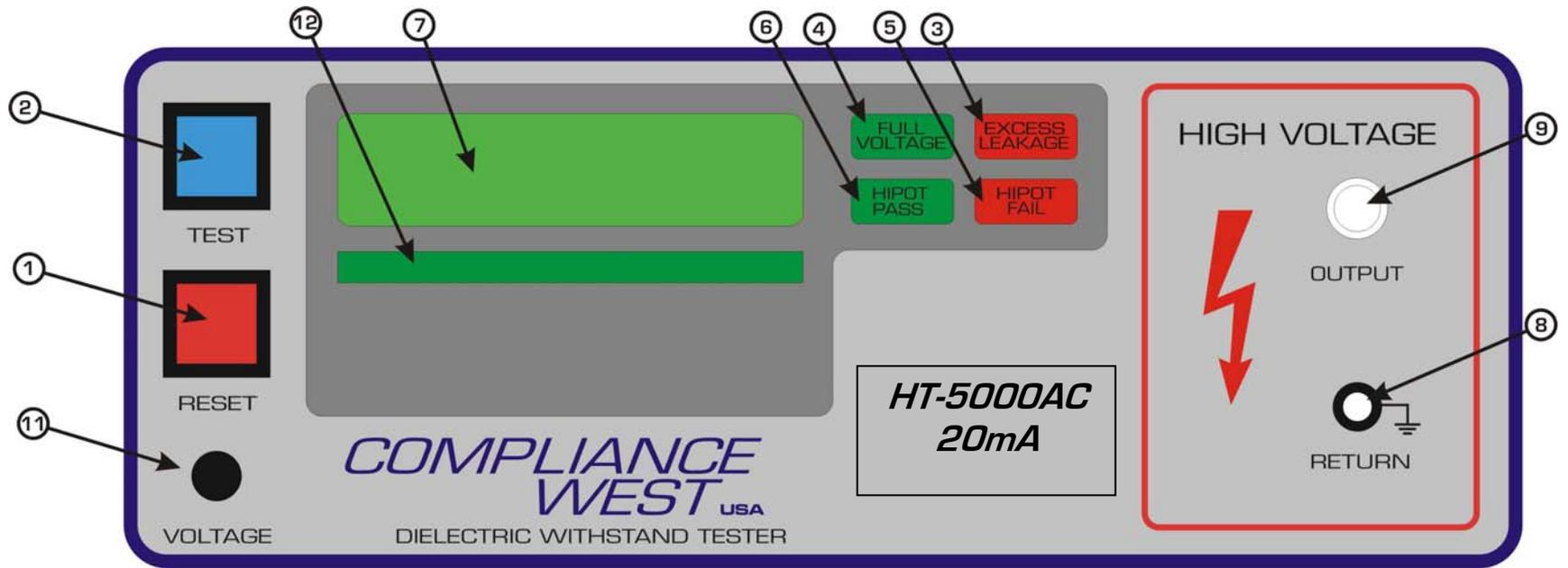
Figure 3-1. Controls, Indicators, Connectors - Model HT-5000ACAC 20mA Front Panel
