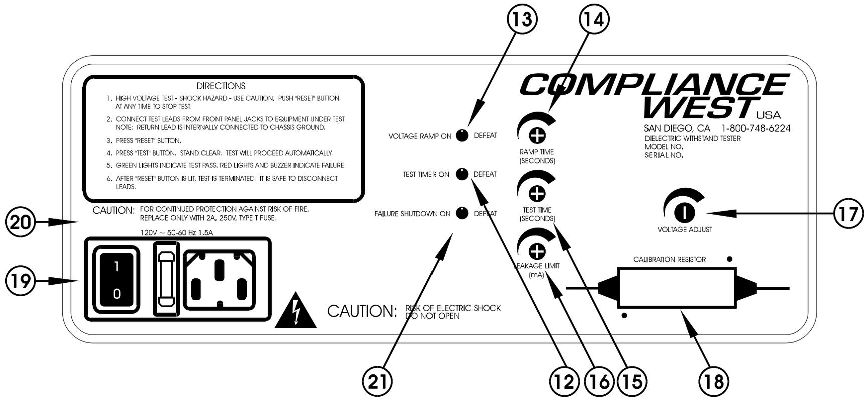
Figure 3-2. Controls, Indicators, Connectors - Model HT-5000ACAC 20mA Rear Panel
