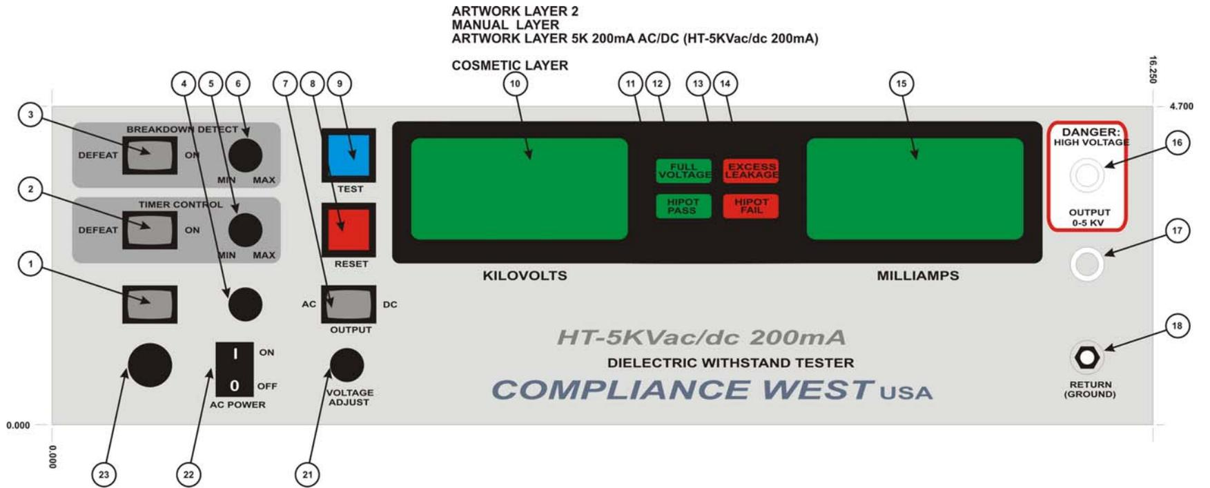
Figure 3-1. Controls, Indicators, Connectors - Model HT-3kVAC Front Panel
