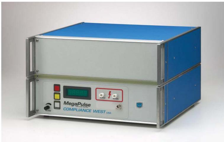
➤ IEC 61010 Surge Tester with 1.2x50/8x20 2 ohm output: 500V - 12kV
