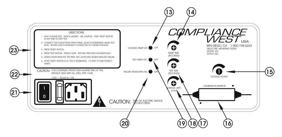
Figure 3. Controls, Indicators, Connectors - Model HT-5000P Rear Panel
