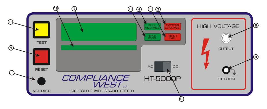
Figure 2. Controls, Indicators, Connectors - Model HT-5000P Front Panel
