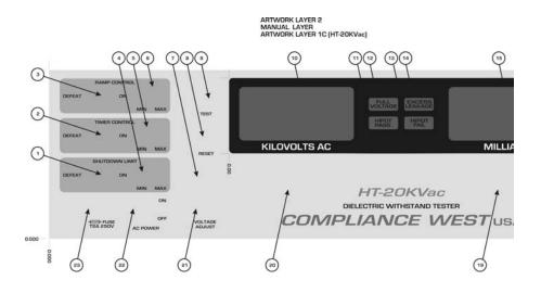
Figure 3-1. Controls, Indicators, Connectors - Model HT-20KVAC Front Panel
