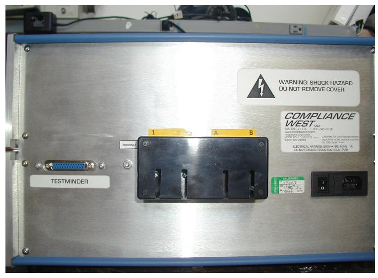
Figure 3 MegaPulse Option Connector Cover
