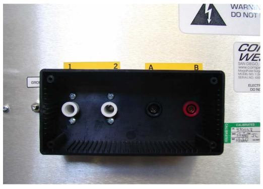
Figure 2 MegaPulse Fast Charge Option Connector
