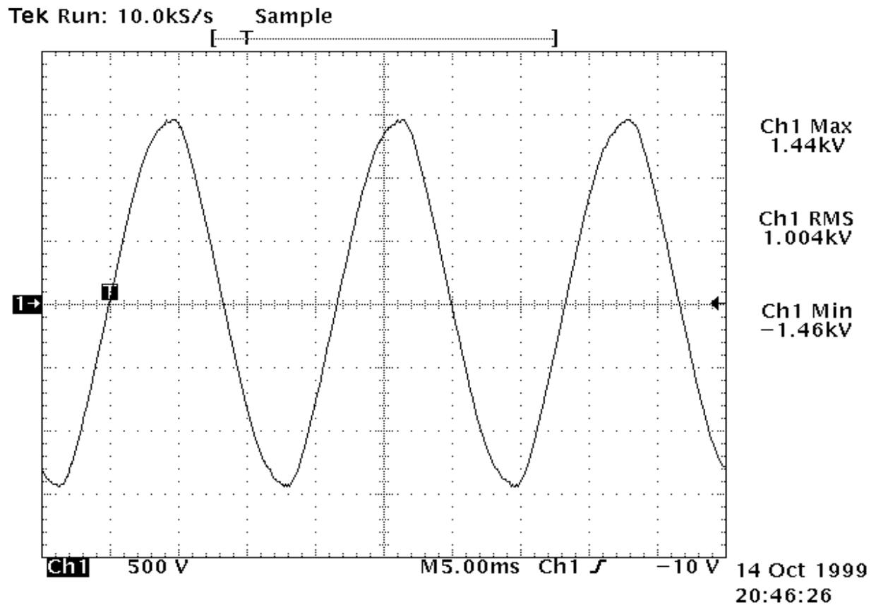
Figure 2 - 1000Vac Waveform
