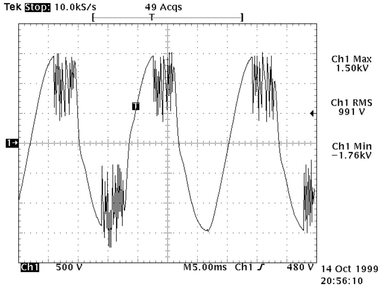
**Figure 4: AC Voltage Dielectric Breakdown**
