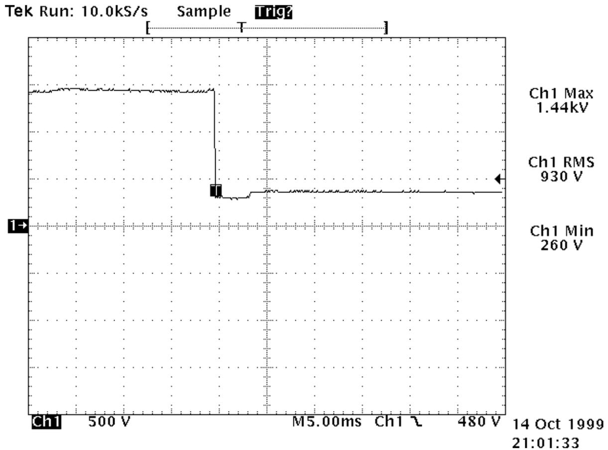
**Figure 5 - DC Voltage Dielectric Breakdown: HT5000 Voltage Shutdown Enabled**
