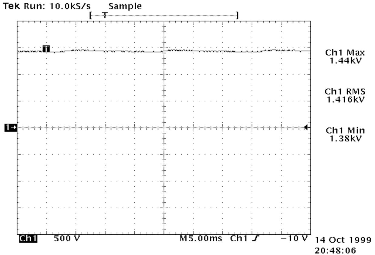
Figure 3 - 1414 Vdc waveform
