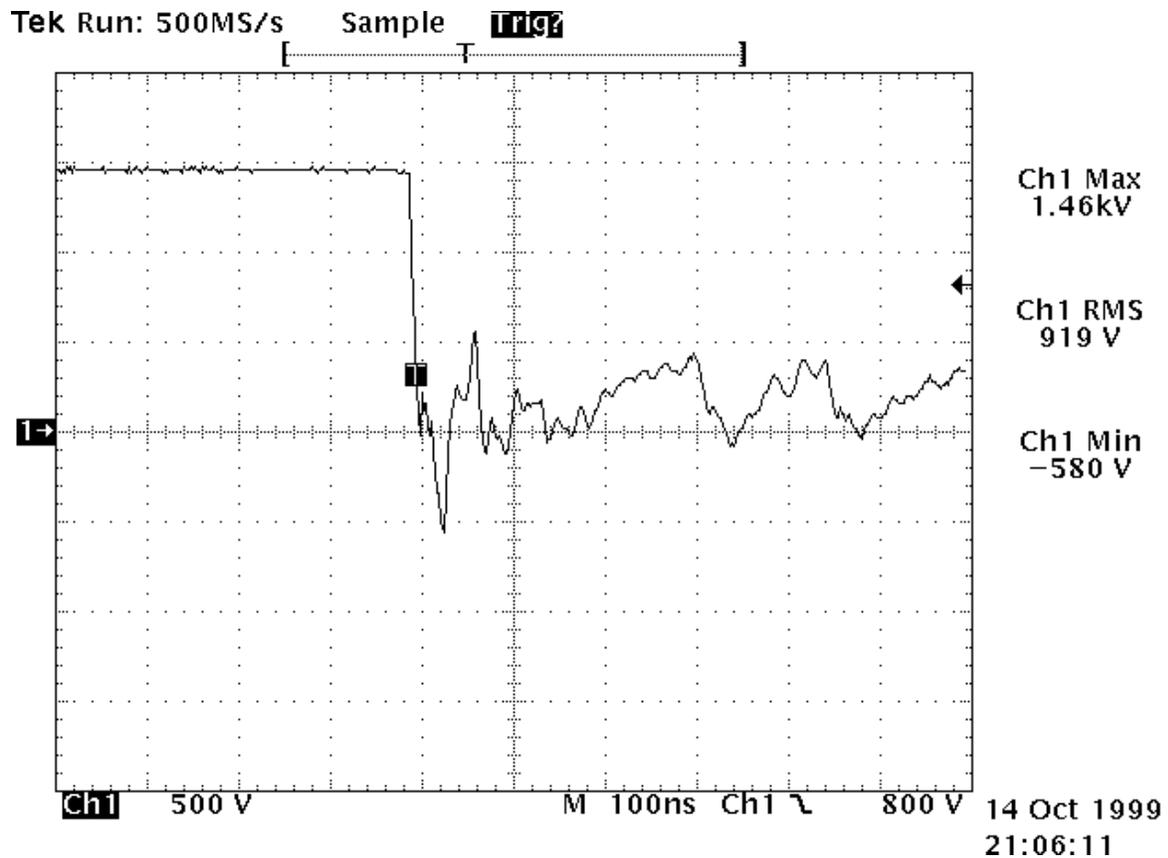
Figure 7 - DC Voltage Breakdown: First 600 ns
