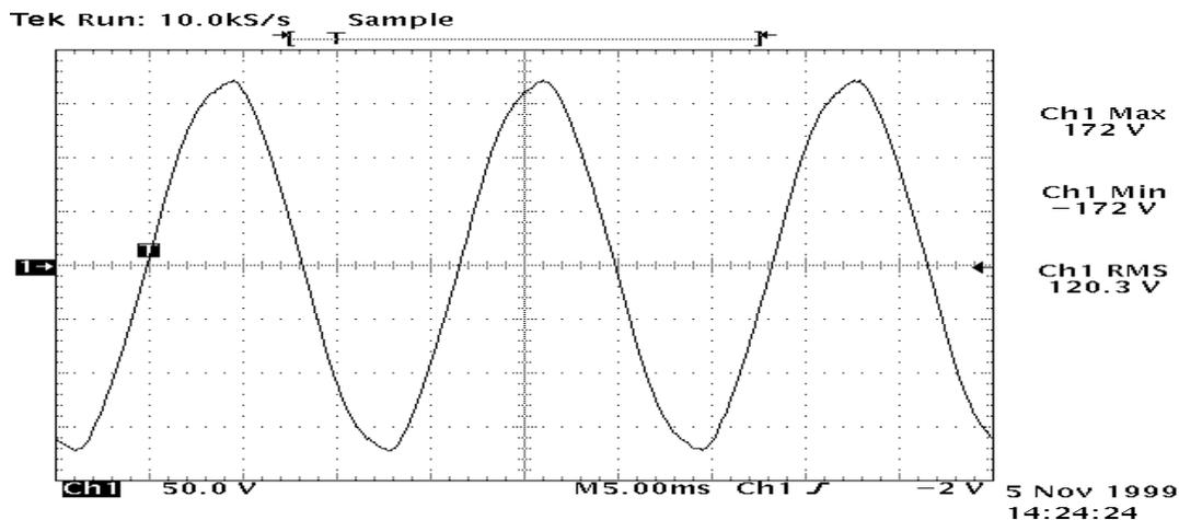
**Figure 1: 120Vac waveform - Wall receptacle power in the U.S.**
